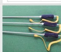
K type thermocouple for tubular furnace
