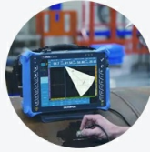
5 Ultrasonic Flaw Detection
