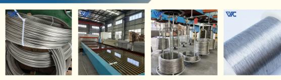
GH4145 wire, also known as Inconel X-750, is a nickel-based high-temperature alloy wire. The material is known for its excellent high-temperature strength, corrosion resistance and heat resistance.
